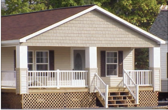
8 FOOT END ELEVATION PORCH WITH WRAPPED POSTS & PVC RAILS (STANDARD ON MODEL 212) 5/12 ROOF PITCH, SHAKER SIDING (CLAY, TAN, WEDGEWOOD OR WHITE)
